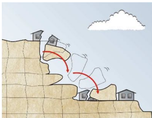
Figure 1 - Failure of an undercut block
